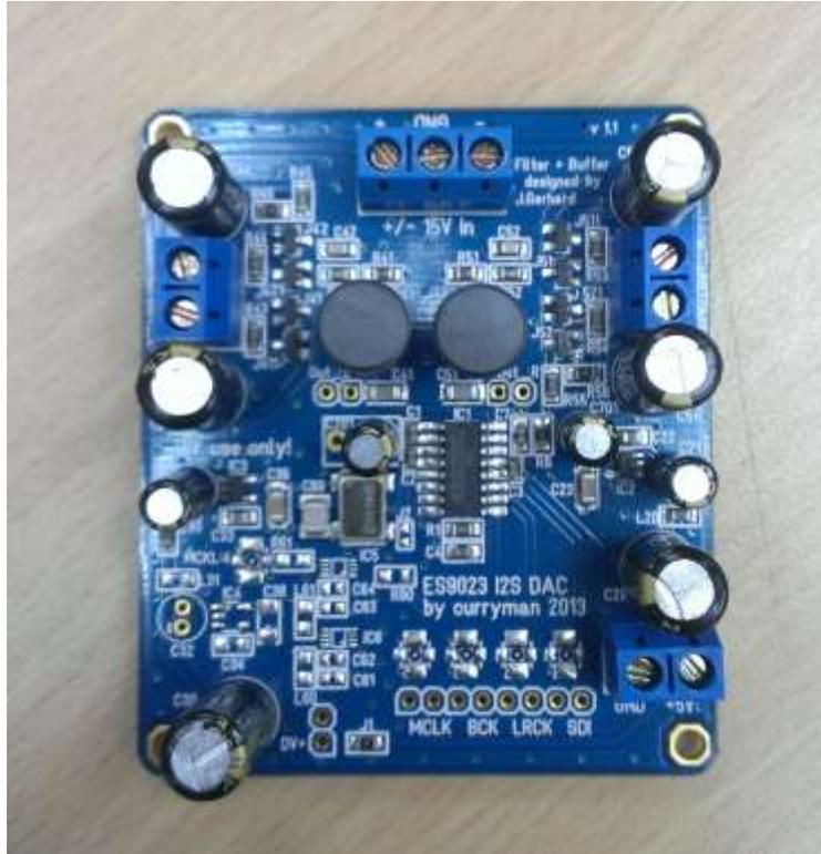
The curryman DAC is a stereo digital to analog converter with I2S input featuring the ES9023 Sabre Premier Stereo DAC and an analog LCR output filter plus JFET buffer (“JG Filter Buffer” developed by Joachim Gerhard) for improved high frequency noise suppression and output drive capability.
