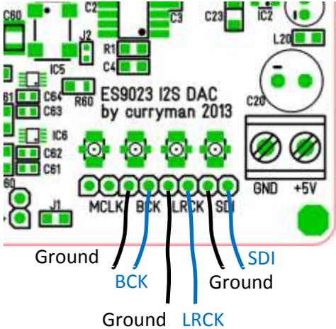
Please keep I2S signal lines as short as possible and provide a separate ground wire for each I2S signal line (e.g. ribbon cable).
